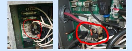
Solution (1): Installing the Power Terminal Block separate from the PC board. If the Power Terminal Block burns due to voltage fluctuations on the power line, the repair can be done by simply replacing a \$20 Power Terminal Block, not the entire PC board for hundreds of dollars.
