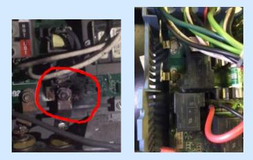
Solution (2): Since 1984 we have used separate and heavy duty contactors to carry the ON/OFF loads of the heaters. Very seldom does a contactor fail; and if it does, since it is separate from the PC board, it only cost \$40 to replace. In addition, all relays are energized at Zero Crossing to minimize electrical spikes.
