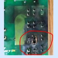
**Solution (4):** We use two separate common relays to operate two water pumps. In addition, all relays are energized at Zero Crossing to minimize the peak load from the motor on the relay contact points.
