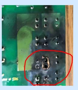
**Solution (4):** We use two separate common relays to operate two water pumps. In addition, all relays are energized at Zero Crossing to minimize the peak load from the motor on the relay contact points.
