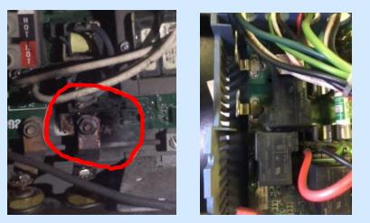
**Solution (2):** Since 1984 we have used separate and heavy duty contactors to carry the ON/OFF loads of the heaters. Very seldom does a contactor fail; and if it does, since it is separate from the PC board, it only cost \$40 to replace. In addition, all relays are energized at Zero Crossing to minimize electrical spikes.
