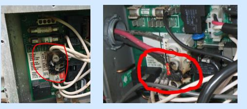
Solution (1): Installing the Power Terminal Block separate from the PC board. If the Power Terminal Block burns due to voltage fluctuations on the power line, the repair can be done by simply replacing a \$20 Power Terminal Block, not the entire PC board for hundreds of dollars.
