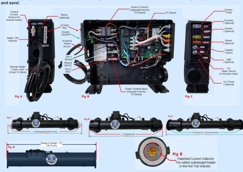
Remote spa heater can be mounted in any position. Connected with 3 foot cables from the control box. Please connect the ground to our ground lug. Can be used with  $\frac{3}{4}$ ", 1", 1 $\frac{1}{2}$ ", 2" water pipe. Can also be used as a low flow heater. You may buy reducer busings 2" to  $\frac{3}{4}$ " from Table 3 or from your local plumbing supply store. For any hot tub installation, connect your existing pipe plumbing (In/Out) to our heater.
