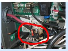
Solution (1): Installing the Power Terminal Block separate from the PC board. If the Power Terminal Block burns due to voltage fluctuations on the power line, the repair can be done by simply replacing a \$20 Power Terminal Block, not the entire PC board for hundreds of dollars.
