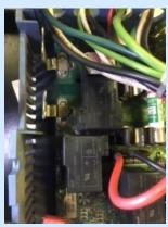
Solution (2): Since 1984 we have used separate and heavy duty contactors to carry the ON/OFF loads of the heaters. Very seldom does a contactor fail; and if it does, since it is separate from the PC board, it only cost \$40 to replace. In addition, all relays are energized at Zero Crossing to minimize electrical spikes.
