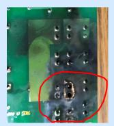
Solution (4): We use two separate common relays to operate two water pumps. In addition, all relays are energized at Zero Crossing to minimize the peak load from the motor on the relay contact points.
