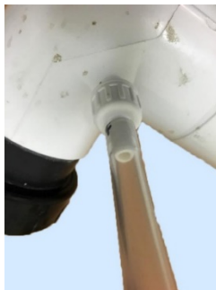
Figure (8) Flex Tube Installed on AABV
