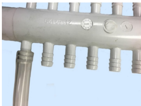
Figure (9) Flex Tube Installed in Air Manifold
