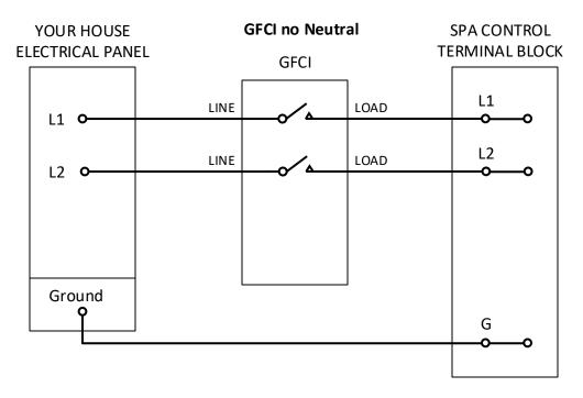
We are DO NOT manufacture GFCIs. Read your GFCI wiring diagram. This diagram is a generic diagram for a properly wired GFCI.
